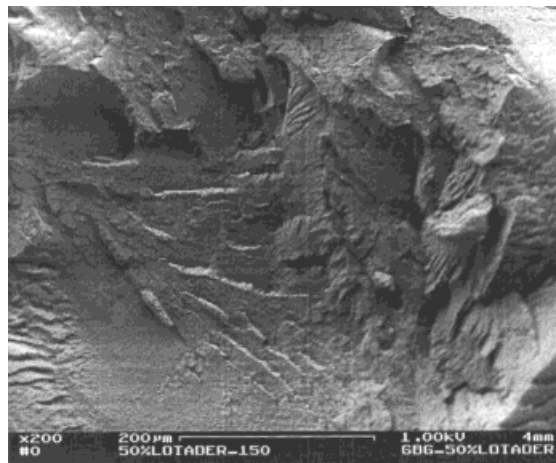
Figure 11 SEM of the blend with 50% PE-F. Magnification \times 200 .
