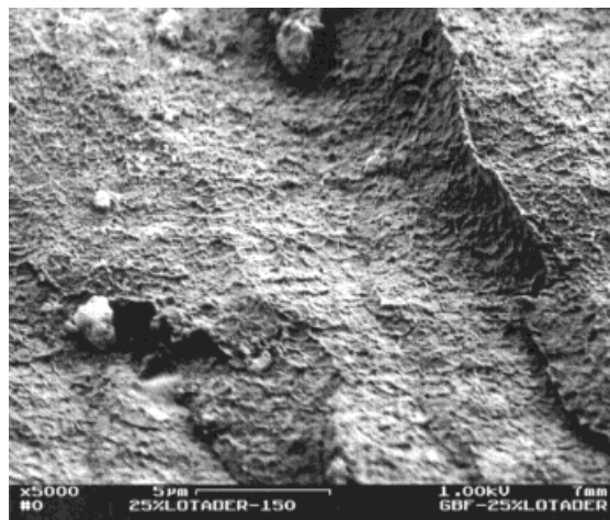
Figure 12 SEM of the blend with 25% PE-F. Magnification \times 5000 .
